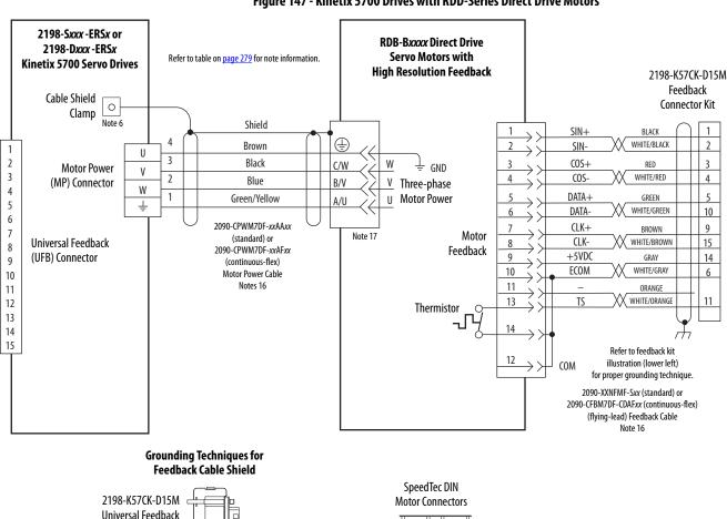
Figure 147 - Kinetix 5700 Drives with RDD-Series Direct Drive Motors
