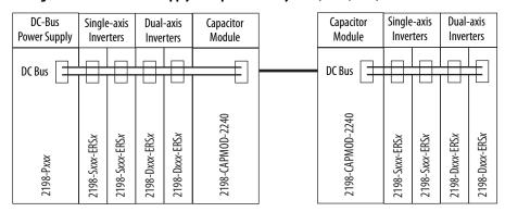
Figure 25 - DC-bus Power Supply Example/Multiple Capacitor Modules (200 A, max)
