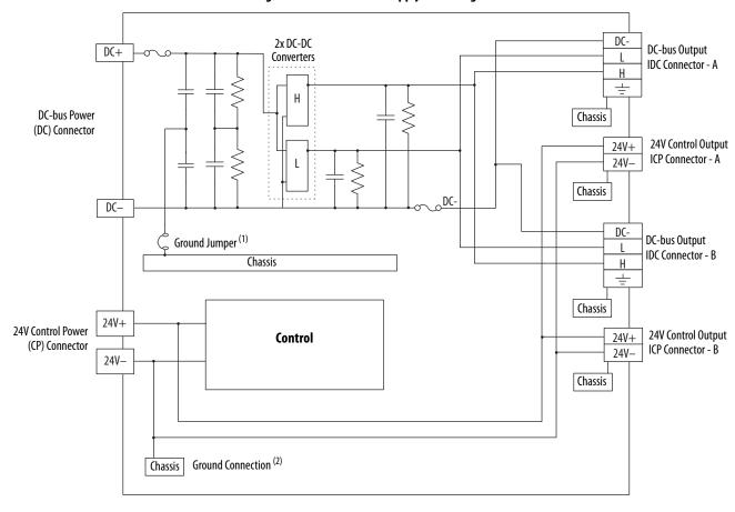
Figure 156 - iTRAK Power Supply Block Diagram
