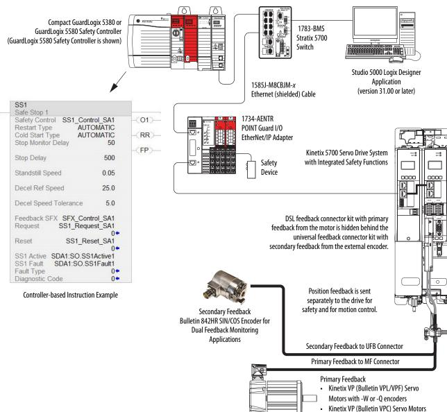
Figure 13 - Safe Motion-monitoring Configuration
