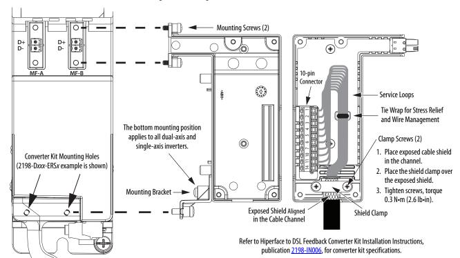
Figure 86 - Wiring the 2198-K57CK-D15M Feedback Connector Kit
