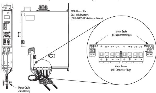
Figure 71 - MP and BC Connector Wiring (dual-axis inverters)
