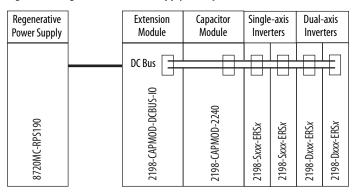
Figure 27 - Multiple DC-bus Power Supply Example/Second System (200 A, max)
