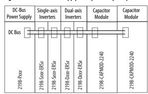
Figure 26 - Regenerative Power Supply Example Power (200 A, max)
