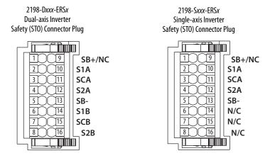
**Table 132 - Safe Torque-off Connector Pinouts**
