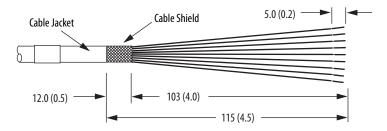
Figure 84 - Lead Preparation for 2198-K57CK-D15M Connector Kit
