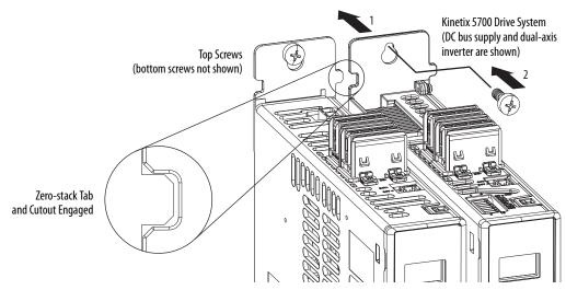
**5.** Attach additional drive modules to the right of the previous module by using the same method, but also making sure that the zero-stack tabs and cutouts are engaged.
