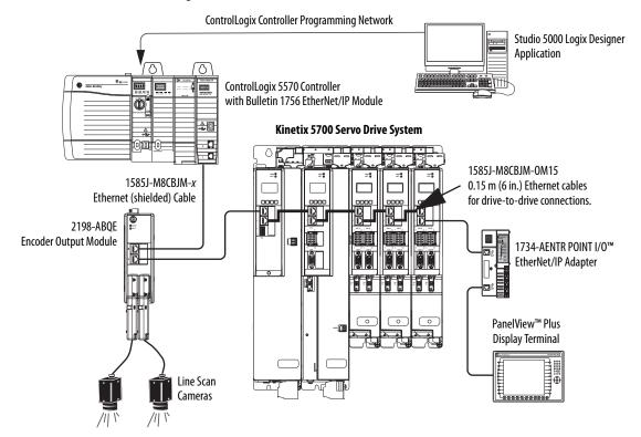
Figure 7 - Kinetix 5700 Linear Communication Installation
