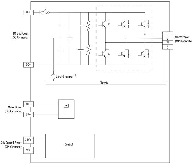
Figure 154 - Single-axis Inverter Block Diagram
