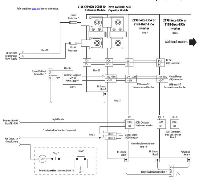
In this example, three-phase AC input power is fed to the 8720MC-RPS190 unit. The DC-bus (TB1) terminals connect to the Kinetix 5700 DC-bus via the 2198-CAPMOD-DCBUS-IO extension module because the system current exceeds 100 A.
