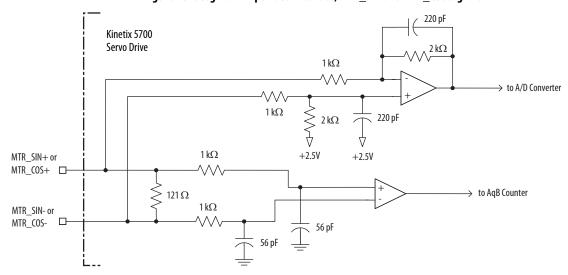
Figure 47 - Stegmann Hiperface Interface, MTR\_DATA Signals
