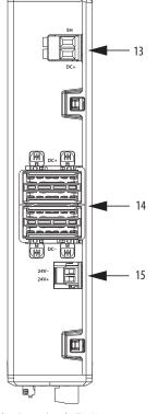
DC-bus Power Supply, Top View (2198-P031 module is shown)
