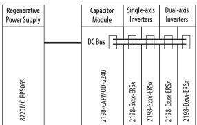
Figure 24 - DC-bus Power Supply Example/Second System (100 A, max)
