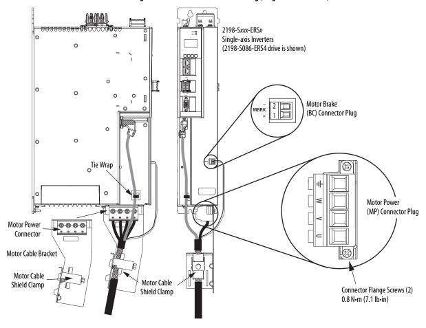
Figure 72 - MP and BC Connector Wiring (single-axis inverters)
