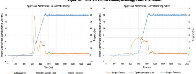
Figure 166 - Effects of Current Limiting on an Aggressive Acceleration
