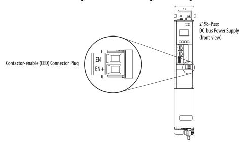
Table 54 - Contactor-enable (CED) Connector Plug Specifications
