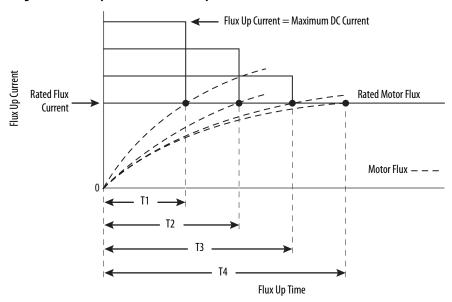
Figure 173 - Flux Up Current versus Flux Up Time
