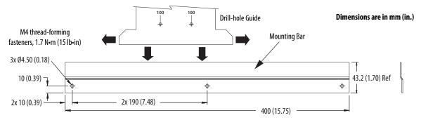
Follow these steps to locate the drill-holes by using the system mounting toolkit.
