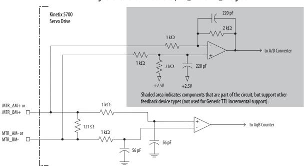
Kinetix 5700 Servo Drive  $1\,\mathrm{k}\Omega$ MTR\_IM+ □ > to AqB Counter 121  $\Omega$ MTR\_IM-56 pF +5V Shaded area indicates components that are part of the circuit, but support other feedback device types (not used for Generic TTL incremental support).  $1\,\mathrm{k}\Omega$ → to UART < from UART \_ 100 pF 100 pF  $1\,k\Omega$ < from UART
