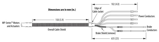
Motor power and brake conductors on 2090-CPBM7DF (series B) 12 and 10 AWG standard, non-flex cables provide (drive end) shield braid and conductor preparation designed for compatibility with multiple Kinetix servo-drive families, including Kinetix 5700 drives.
