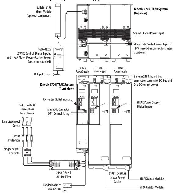
Figure 5 - Typical iTRAK Power Supply Installation
