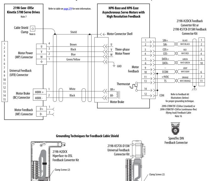
Figure 146 - Kinetix 5700 Drives with HPK-Series Rotary Motors
