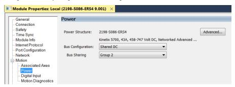
Figure 101 - Group 2 Dual-axis Inverter Configuration
