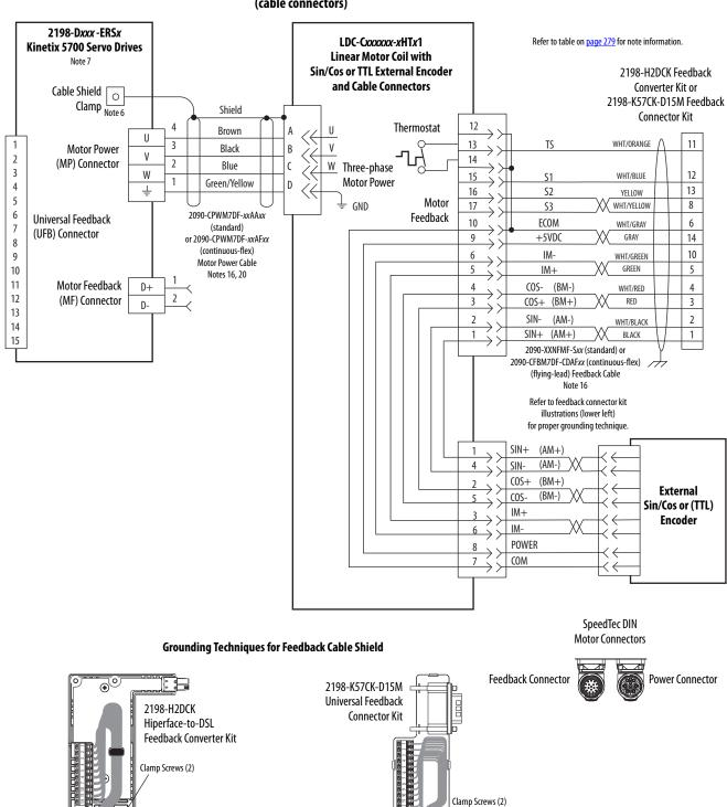
Figure 151 - Kinetix 5700 Drives with LDC-Series Linear Motors (cable connectors)
