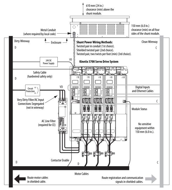
Observe these guidelines when mounting your 2198-R004 external passive shunt resistor:
