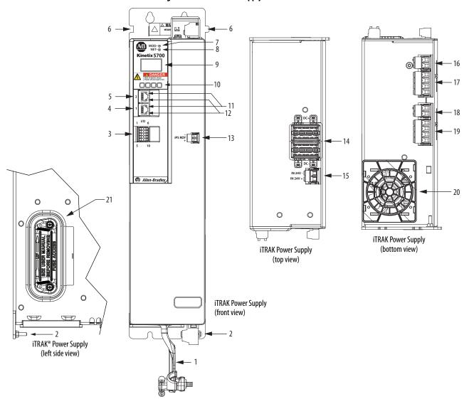
Figure 37 - iTRAK Power Supply Features and Indicators
