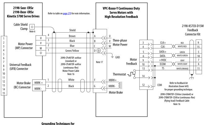
Figure 144 - Kinetix 5700 Drives with Kinetix VP Continuous Duty Motors
