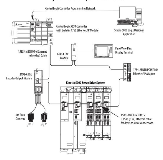
Figure 8 - Kinetix 5700 Ring Communication Installation
