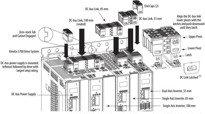
Figure 29 - DC-bus Connector Example
