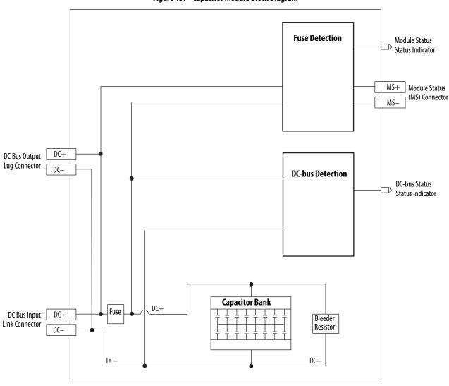
Figure 157 - Capacitor Module Block Diagram
