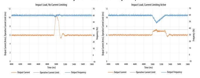
Figure 167 - Effects of Current Limiting on an Impact Load
