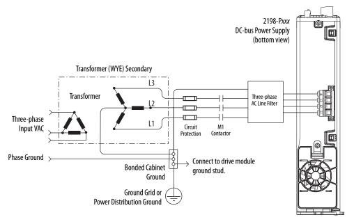
2198-Pxxx **DC-bus Power Supply** (bottom view) Transformer (WYE) Secondary L3 Transformer Three-phase L1 Circuit Input VAC Protection Contactor Phase Ground Connect to **Bonded Cabinet** drive module Ground ground stud. Ground Grid or **Power Distribution Ground**
