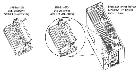
Table 133 - Safe Torque-off (STO) Connector Plug Wiring
